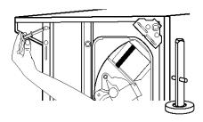
**STEP 3.** Check adjustability of rear legs, by pushing in one leg. The other leg should come out. Check both legs. If they do not adjust, repeat STEP 2.
